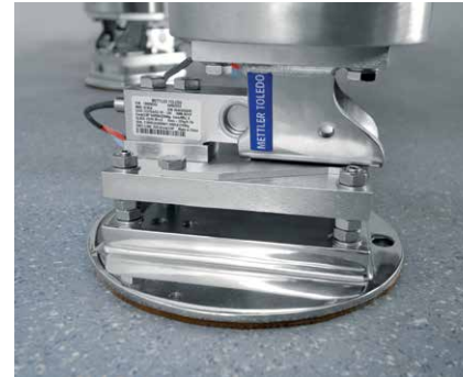
Weighing cell in one of the feet of the vessel, along with its corresponding section in the software program, essential components of the automatic dosing system.
