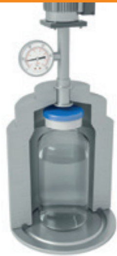
Pressure decay method (P)
