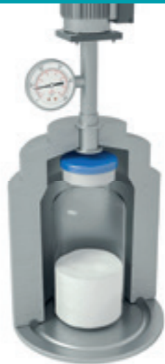
Vacuum decay method (V)
